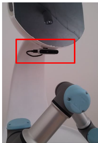
Figure 4. The RGB-D camera used in image acquisition located at a mobile robot manipulator.
